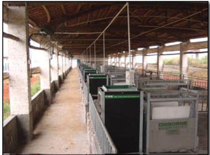
The FIRE System automates the measurement and collection of individual animal feed intake and growth performance. Each individual pig is tagged with a Radio Frequency Identification (RFID) tag and the tag is read by an antenna located in the FIRE Feeder, and feed intake and animal weight are recorded.
