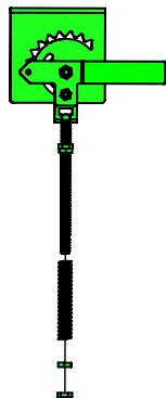
15. Place feed flow control onto crossbar with back side of assembly resting against flat side of crossbar. Install the feed flow control to crossbar with 5/16 x 7/8-in. bolt and 5/16-in. flange nut.
