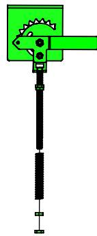
15. Place feed flow control onto crossbar with back side of assembly resting against flat side of crossbar. Install the feed flow control to crossbar with 5/16 x 7/8-in. bolt and 5/16-in. flange nut.
