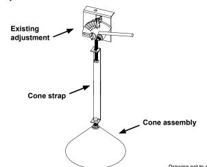
Replace cone strap and cone assembly on the axle inside feeder.
