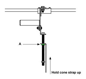
6. Slide feed flow control spring onto bolt from the bottom up. Thread nuts (C & D) behind it.
