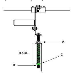
While holding a wrench on nut (A), tighten nut (C) to tension the spring to a length of 3.5-in. Tighten nut (D) against nut (C).
