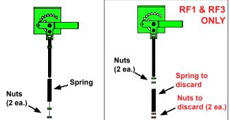
For Model RF1 (7.5 bu) and RF3 (15 bu), remove all nuts (4 ea.) and spring. Discard two (2) nuts and spring. These parts will not be used and may be discarded.
