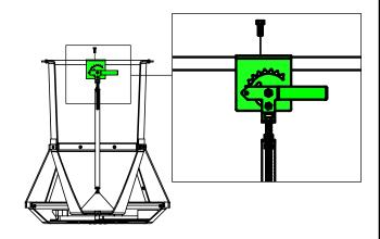
Install using 5/16 x 7/8-in. bolt and 5/16-in. nut removed in previous step.
