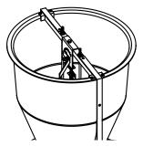
Place the feeder in the fenceline between two properly spaced posts or other immobile objects. Attach the adapters to the fenceline using the holes provided.
