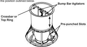
NOTE: Some older feeders are not equipped with pre-punched slots. The fenceline adapter frame can be used as a guide for drilling holes into correct trough divider bars.
