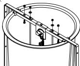
Attach fenceline adapter outer frame to penning or other immobile object. FOR DROP ROD FENCELINE ADAPTERS, CONTINUE ASSEMBLY WITH STEP 5 ON REVERSE SIDE.
