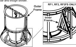
NOTE: For fenceline adapters for feeder models RF1, RF2, and RF2FS, an inner angle must be installed WITH outer frame as shown. Refer to Step 3.
