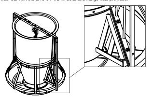
Attach top of fenceline adapter outer frame to crossbar's outer holes using the 5/16 x 7/8-in. bolts and nuts provided. Repeat Steps 1-4 for other fenceline adapter. After fenceline adapters have been installed, reinstall bump bar agitators (if applicable).
