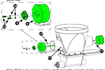
Slide PVC guide cap on agitator shaft assembly and into plastic guides. Secure cap to plastic guide through the pre-drilled holes in the guide using two (2) #14 x 1-in. self-drilling screws (Item 17) and 3/8 socket. Repeat process for second PVC guide cap.
