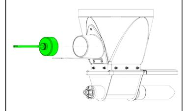
**IMPORTANT NOTE:** Use hole saw in a counter-clockwise direction to allow for smoother cutting.
