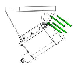
4. Using a 1-1/2-in. hole saw, drill a hole into the upper boot/plastic transition using the upper agitator guide as a guide.
