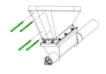
7. Assemble the motor mount plate (Item 2), agitator guide (Item 8), spacer (Item 9), if required, and half gaskets (Item 21) as shown using four (4) 1/4 x 1-3/4-in. bolts (Item 14) and 1/4-in. rubber wellnuts (Item 15).
