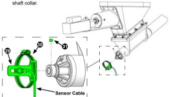
Install the feed delivery system sensor (included with Item 12) onto the sensor mounting bracket using the nuts included on the sensor. Adjust the position of the sensor on the mounting bracket until it aligns with the magnet and is within approximately 1/4-in. of the magnet. Gently tighten the nuts on the sensor with a 1/2-in. wrench.
