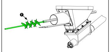
NOTE: For bins with feed, sliding a 3/4 to 1-in. ID pipe through the opposite end of the boot and over the shaft assembly to guide the assembly through the feed may allow for easier installation.
