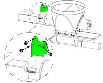
Attach gate slide sensor (included with Item 9) to gate slide using the 3/8-in. cable clamp (Item 32) and #10 x 3/4-in. self-drilling screw (Item
