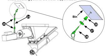
Loop motor support cable (Item 24) through grommet hole on motor/cable mounting bracket and secure cable using cable clamp (Item 25). Loop opposite end of motor support cable through eye bolt and secure using second cable clamp (Item 25). Ensure there is no slack in the cable and motor is fully supported, then cut and discard excess cable leaving a 6-in. "tail" at each end.
