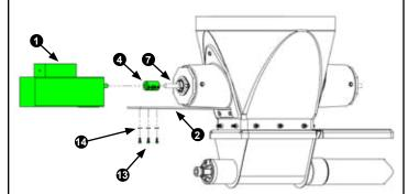
Adjust coupling and agitator shaft until both shafts extend approximately half-way through the coupling. Fully tighten bearing mounting plates installed in previous step with a 7/16-in. socket and the set screw in the bearings using a 3/32-in. hex key. Then, tighten the bolts in the shaft coupling using a 9/64-in. hex key.
