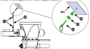
Loop motor support cable (Item 20) through grommet hole on shaft safety cover/cable mounting bracket (Item 3) and secure cable using cable clamp (Item 21). Loop opposite end of motor support cable through eye bolt and secure using second cable clamp (Item 21). Ensure there is no slack in the cable and motor is fully supported, then cut and discard excess cable leaving a 6-in. "tail" at each end.
