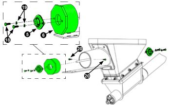
Slide PVC guide cap on agitator shaft assembly and into lower plastic guide. Secure to plastic guide using two (2) #14 x 1-in. self-drilling screws (Item 20) and 3/8 socket.
