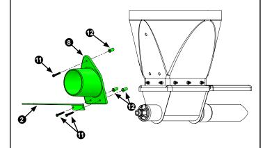
4. Install two (2) half gaskets (Item 18) around back opening of the agitator guide (Item 8) and attach the agitator guide and motor mount assembly to the upper boot/plastic transition.
