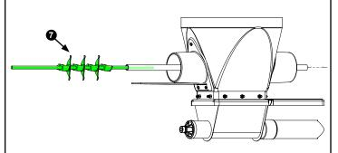
NOTE: For bins with existing feed, slide a 3/4 to 1-in. ID pipe through the opposite end of the boot and over the shaft assembly to guide the assembly through the feed for easier installation.
