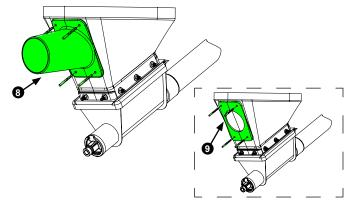
NOTE: A plastic spacer (Item 9) is provided for installation on certain boots where plastic agitator guides do not fit the contour of upper boot/plastic transition. Use spacers as drilling guide in these cases.
