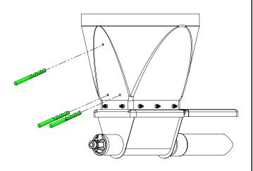
3. Assemble the agitator guide (Item 8) and motor mount plate (Item 2) as shown using three (3) 1/4 x 1-3/4-in. bolts (Item 11) and 1/4-in. rubber wellnuts (Item 12).
