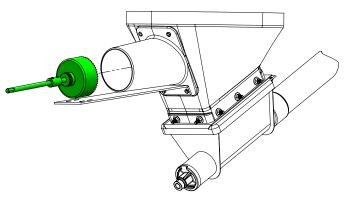
**IMPORTANT NOTE:** Use hole saw in a counter-clockwise direction to allow for smoother cutting.
