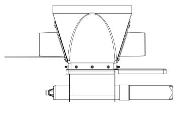
7. Insert the agitator shaft assembly (Item 7) into the upper boot/plastic transition through the plastic guides.
