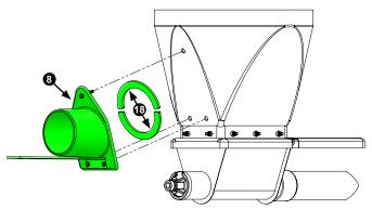
5. Using a 4-3/8-in. hole saw, drill a hole into the upper boot/plastic transition using the agitator guide as a guide.
