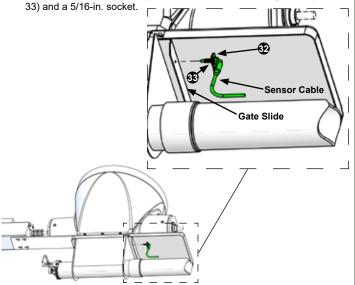
13. Remove paper backing and attach the magnetic strip (Item 34) to the bottom of the slide cover, aligning it with the gate slide sensor. Ensure the magnetic strip is located such that the gate slide sensor can detect it when the gate slide is fully open.
