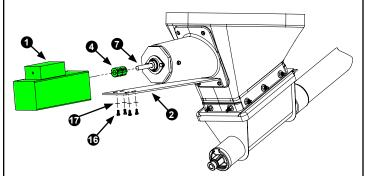
Adjust coupling and agitator shaft until both shafts extend approximately half-way through the coupling. Fully tighten bearing mounting plates installed in previous step with a 7/16-in. socket and the set screw in the bearings using a 3/32-in. hex key. Then, tighten the bolts in shaft coupling using a 9/64-in. hex key.
