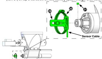
Install feed delivery system (auger) sensor (included with Item 9) onto sensor mounting bracket using the nut included with the sensor. Adjust the position of the sensor on the mounting bracket until it aligns with the magnet and is within approximately 1/4-in. of the magnet. Gently tighten the nuts on the sensor with a 1/2-in. wrench.
