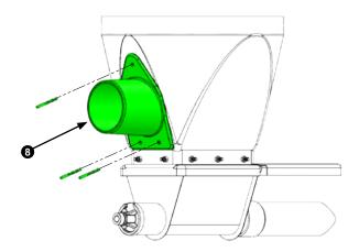
2. Remove the agitator guide (Item 8) and enlarge the holes in upper boot/ plastic transition using a 1/2-in. drill bit.
