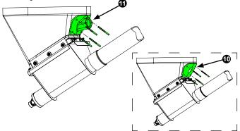
NOTE: A plastic spacer (Item 10) is provided for installation on certain boots where the plastic agitator guides do not fit the contour of the upper boot/plastic transition. Use spacers as drilling guide in these cases.
