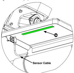
Attach the gate slide sensor (included with Item 12) to the gate slide using the 3/8-in. cable clamp (Item 32) and #10 x 3/4-in. self-drilling screw (Item 33) and a 5/16-in. socket.
