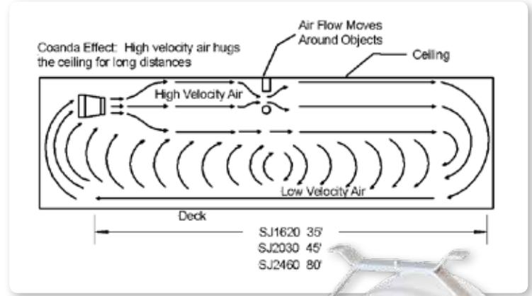
**High jet velocity** creates a jet-stream of beneficial air movement far greater than the Super-Jet's own output, as shown above. Proper mixture means fresh air is uniformly available—"dead air" is eliminated!
